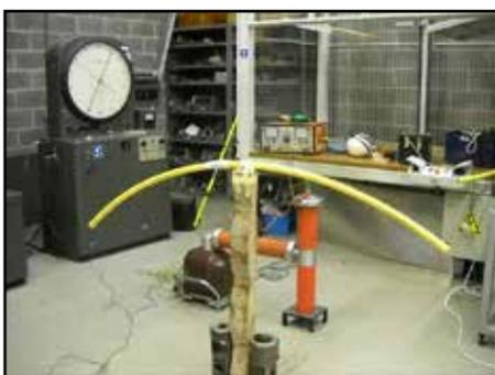
The picture shows a setup of a dielectric test of the LPG-Flex® pipe by a third party lab to meet the new EN 16125 Standard.
