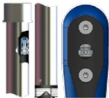
Air transfer valve in the drop tube. Air in the fill line escapes into the tank ullage at the start of the filling operation
